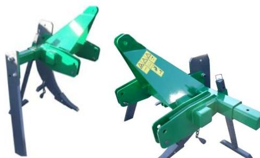
Fig. 5. Scarifier GZ/P with tree root cutter [6]
