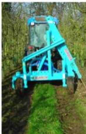
Fig. 4. Equipment for shaping tree roots, AGROFER [5]
