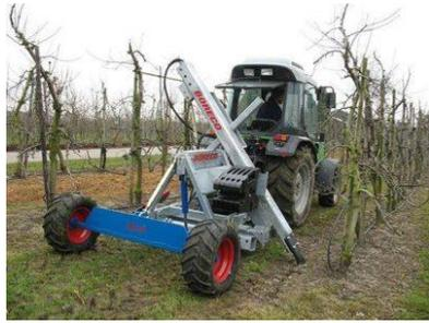
Fig. 6. Device for shaping tree roots, BORECO [7]
